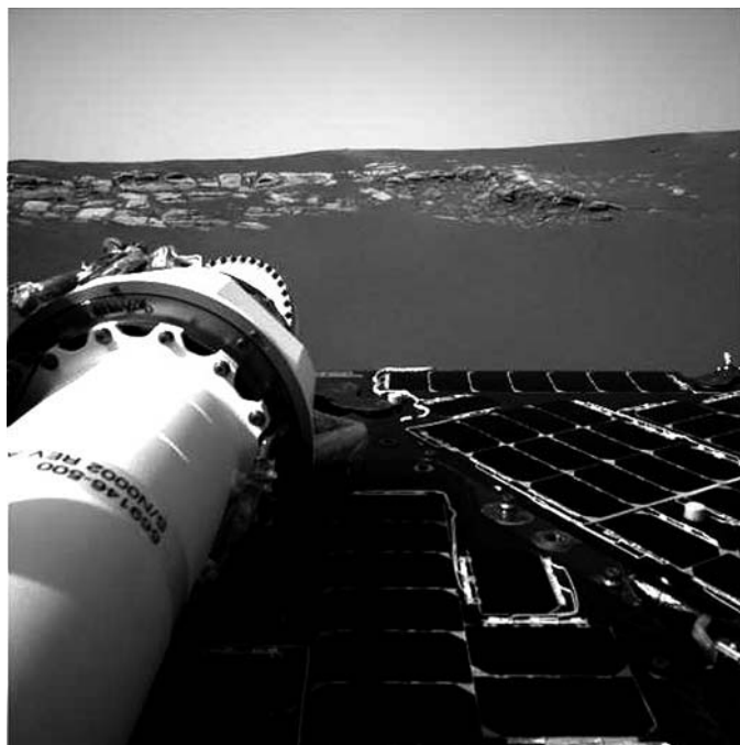
Fig. 1. The first image of the martian surface acquired by Opportunity. It is a Navcam image acquired on sol 1, reduced in resolution to 512 \times 512 pixels and obtained before deployment of the Pancam Mast Assembly. (Image ID = 1N128285132.)
